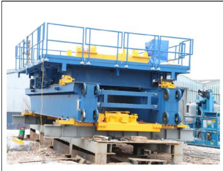
Main Frame & Cross Travel Carriage
